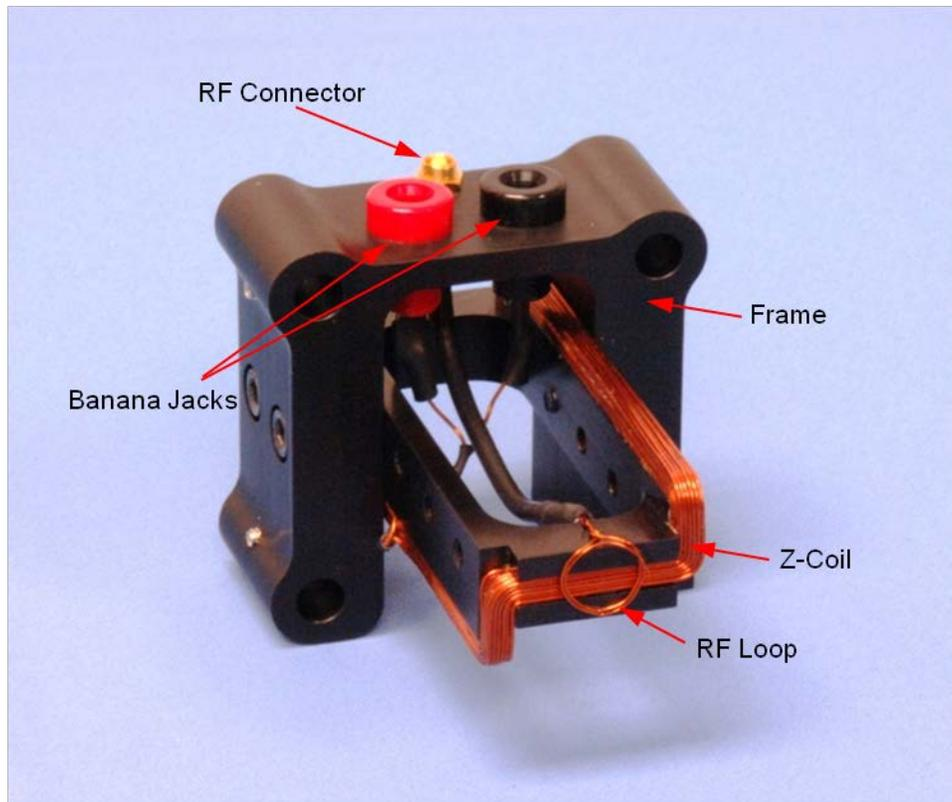
Figure 1: Photograph of the Z-coil and RF loop assembly.
