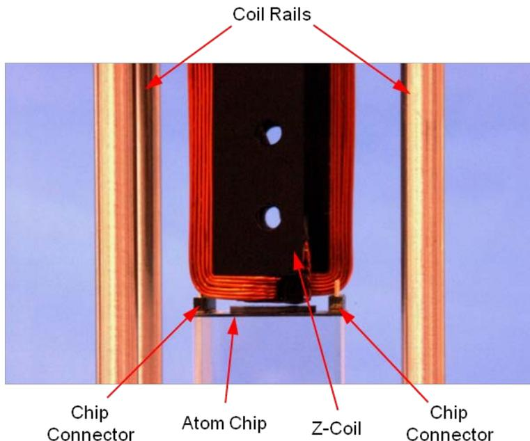
Figure 2: Photograph of the Z-coil mounted on the coil rails, and its position relative to the atom chip. Not shown are the 3D coil assembly and flex wires that connect to the atom chip.
