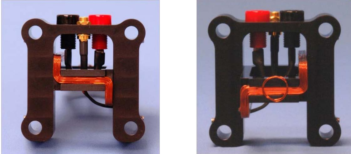
Figure 3: Top (left) and bottom (right) view of the Z-coil. The assembly can be mounted upside down to change the sense of the "Z."
