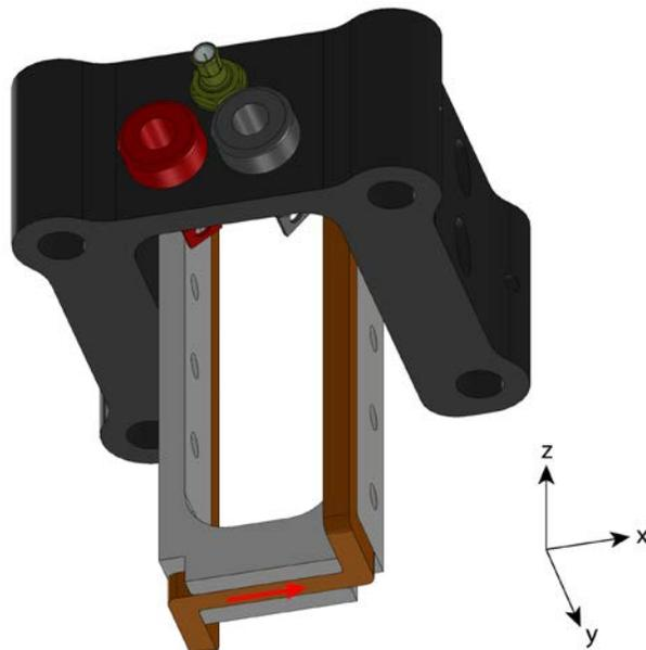
Figure 4: When mounted in the orientation shown in Figure 3, a positive current creates a magnetic field underneath the coil that points in the +y direction (away from the front of the banana jacks). For simplicity, the RF loop is not shown.
