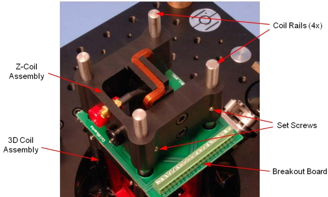
Figure 5: Top view of the installed Z-coil assembly. The assembly bolts onto the four coil rails via four set screws and rests above the breakout board and 3D coil assembly.
